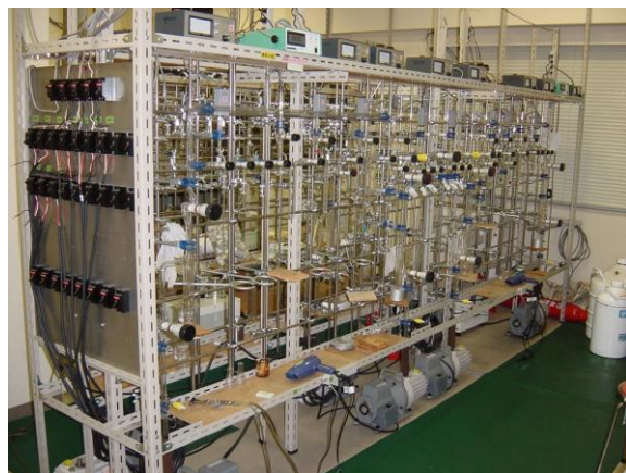
Figure 4.14 Photo of glass-line vacuum system used for sample preparation.
