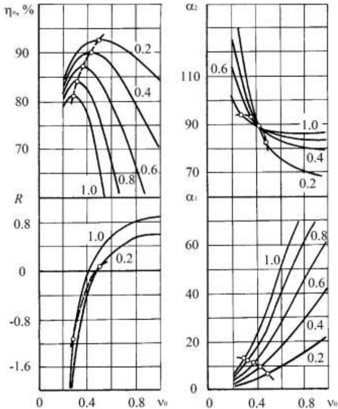
**Figure 3.5** Optimal characteristics of the turbine stage ( $\phi^2 = 0.96$ ,  $\psi^2 = 0.9$ ).
