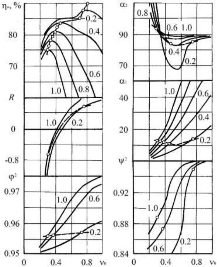
**Figure 3.6** Optimal characteristics of the turbine stage with velocity ratio, calculated by the formula (3.26). The numbers refer to  $\bar{c}_{0z}$  values. Circles mark the optimal parameters at optimal heat drop in the stage.
