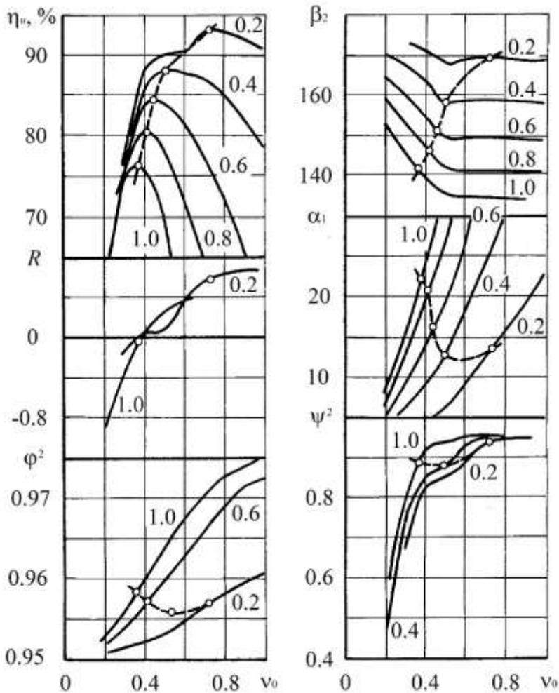
*Figure 3.7 Optimal characteristics of the turbine stage ( $\varphi$ ,  $\psi$  calculated by the formula (3.26)) with  $\psi$  recalculated according to (3.27). The numbers refer to  $\bar{c}_{0z}$  values. Circles mark the optimal parameters at optimal heat drop in the stage.*
