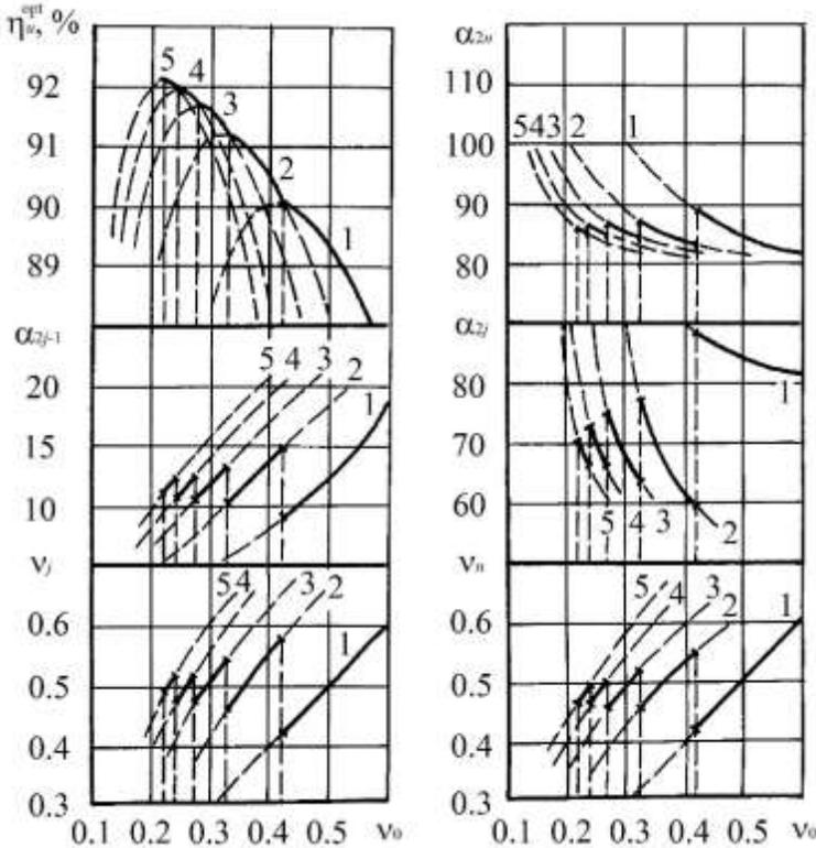
**Figure 3.4** The calculated optimal exit flow angles  $\alpha$ , velocity ratios  $v$  of intermediate and last stages, module efficiency  $\eta$  for different values of the heat drops ( $\bar{c}_{0z} = 0.4$ ,  $\phi^2 = 0.96$ ,  $\psi^2 = 0.9$ ,  $K_{out} = 0.1$ ; ( $j = \overline{1, n-1}$ )). The numbers on the curves indicate the number of stages in the module. The bold line shows the envelope of the parameters, corresponding to the maximum efficiency.
